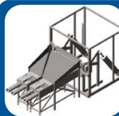
Hoist feeding two stuffers, exiting to the front.
